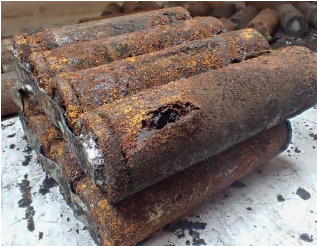
Photo 3: Failed 18650 battery cell
